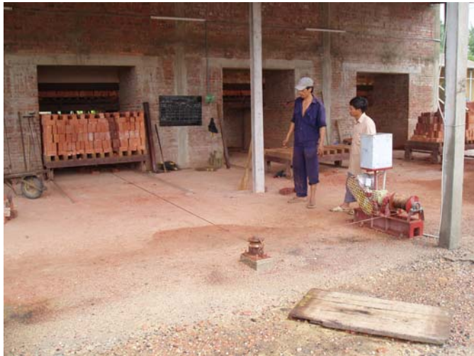
Winch to pull trolley
